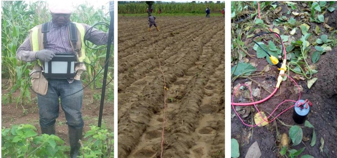
Plate no 1: Magnetic and Induced polarization and resistivity data acquisition
